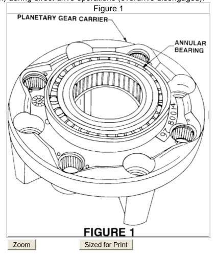
This condition may be caused by a worn annular bearing on the planetary gear carrier (see illustration). Continued operation of a noisy transmission in the direct drive mode will cause damage to the planetary carrier, adapter plate, input sun gear, and input sun gear oil seal. If the input sun gear oil seal is damaged, it is possible for overdrive unit oil (Dexron II) to leak into the manual portion of the transmission.
